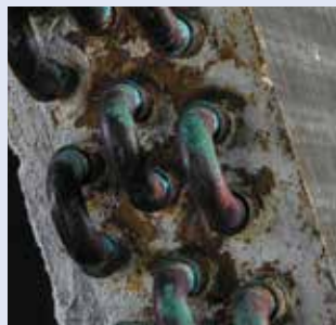
Copper tube and galvanized steel tube sheet after 500 hour salt spray.
